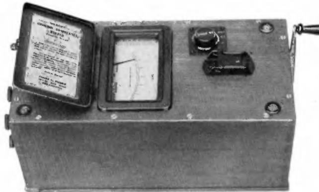
FIG. 6. The heavy-duty type of "Megger" Ground Tester, top view. Approximate dimensions—14x7x7 inches. See facsimile scale, FIG. 21, page 39.
