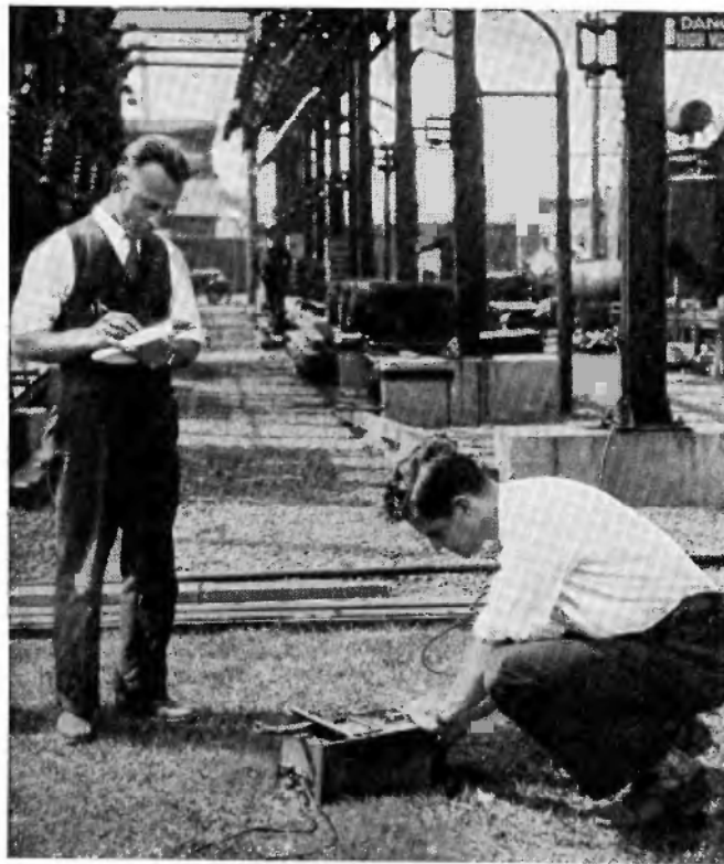
FIG. 2. Testing ground resistance is done with minimum of effort with the "Megger" Ground Tester.
