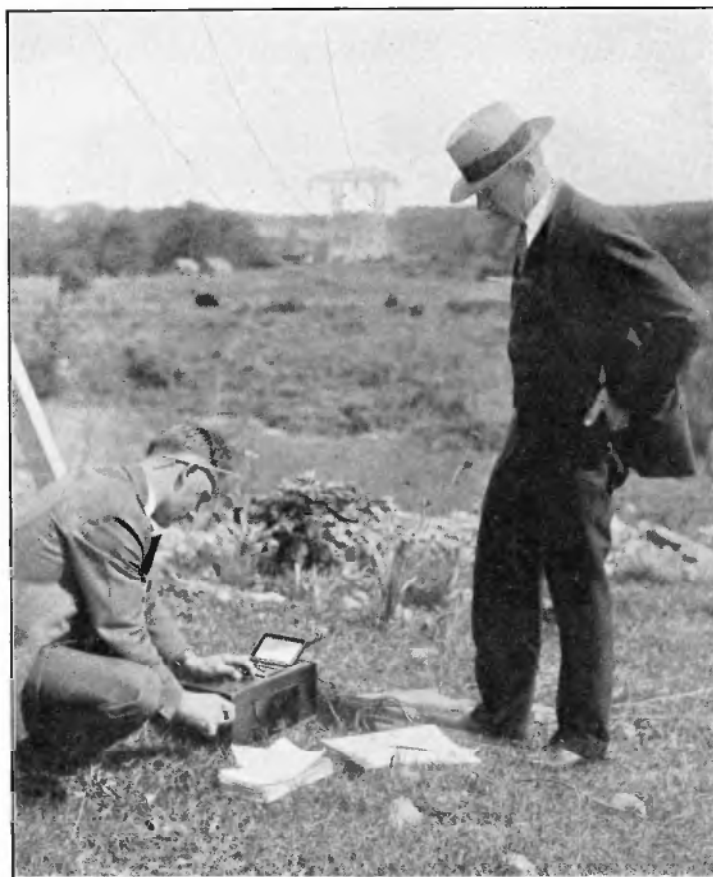
FIG. 29. Testing the resistance to earth of a 220-KV transmission tower, using the "Megger" Ground Tester.
