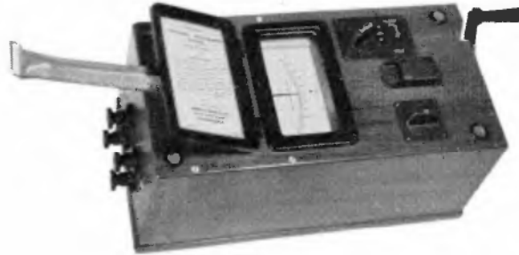
FIG. 37. The low resistance type of "Megger" Ground Tester.
